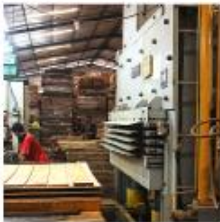
7. LAMINATING PROCESS Top, core and bottom layers are laminated
