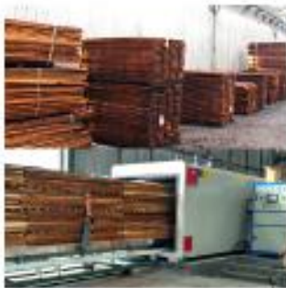
4. KILN DRY PROCESS Each logs then dried ( Kiln Drying ) based on Moisture Content Order
