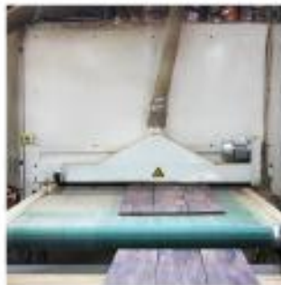
8. SANDING PROCESS Each floors are sanded for smoother surface
