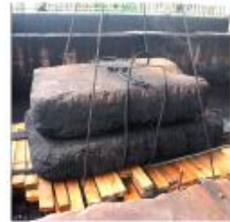
3. ANTI BUG TREATMENT To kill insects inside the timber
