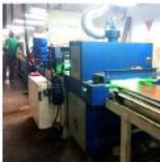
10. COATING Each planks are coated with natural or color staining
